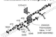
For 1-1/4" Thermostatic Valve (p/n 1621).
