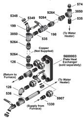
For domestic water heaters using Plate Heat Exchanger (p/n 5600003).
