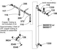
Used to install the Water-to-Water Heat Exchanger (p/n 5600018 or 5600017) on existing domestic water heater for thermal circulating heat transfer. Water-to-water heat exchanger is sold separately.
