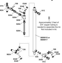
Used to install the Water-to-Water Heat Exchanger (p/n 5600018 or 5600017) on existing domestic water heater for thermal circulating heat transfer. Water-to-water heat exchanger is sold separately.
