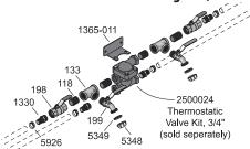
For 3/4" Thermostatic Valve (p/n 2500024).
