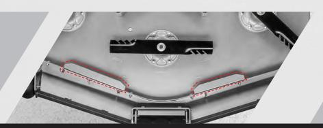
Our exclusive Aero Deck™ is .270-inch fabricated steel and features fully adjustable baffles enabling you to customize your cut to various grass conditions.
