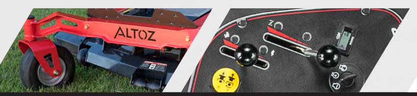
Formed, laser-cut and welded heavy-gauge steel frame for maximum strength and rigidity.
